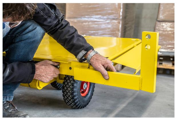
STEP 08: Put the clamp back on and put the pin back in
