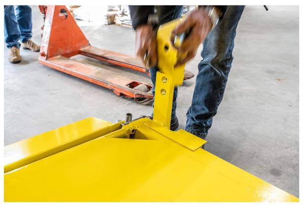
STEP 06: Undo the screws of the normal handel
