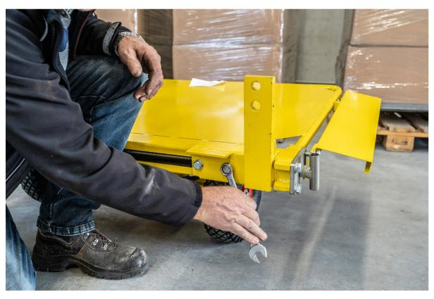
STEP 07: Put the extension arm in place and put the scews back in
